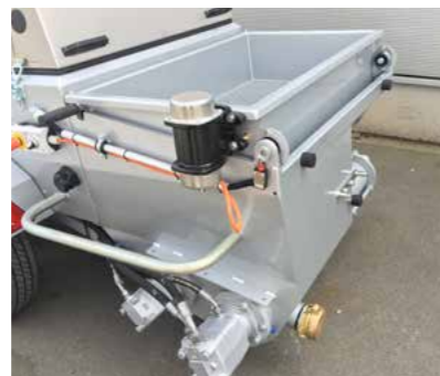
The 400 l mixing vessel
