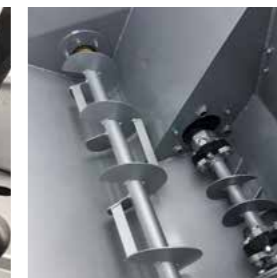
Additional agitator shaft in the hopper
